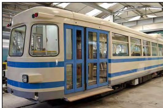
Figure 3-10: FEVE Hydrogen Fuel Cell Streetcar
