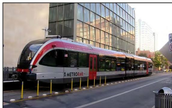
Figure 3-12: Austin, TX Diesel-Electric LRT (Stadler)
