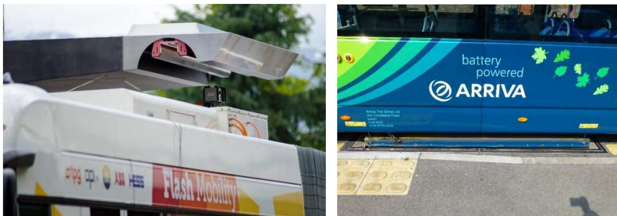
Figure 3-17: ABB Energy Transfer System (left) and Arriva Streetlite EV Bus Charging Plate (right)
