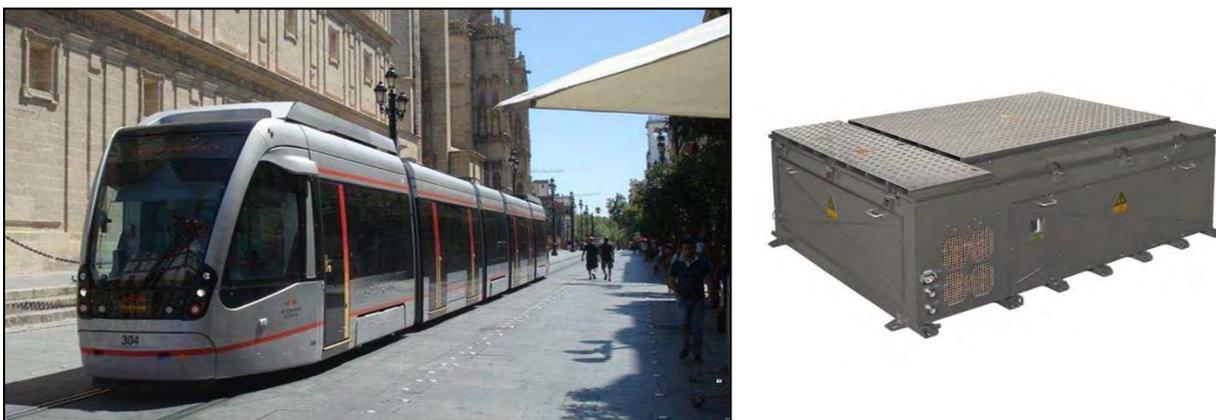
Figure 3-5: CAF Streetcar in Seville, Spain (left); CA Supercapacitor (right)
