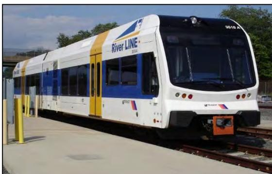
Figure 3-11: New Jersey Diesel-Electric LRT (Stadler)
