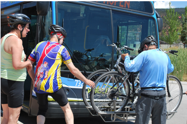
All of RFTA's valley buses have front-load racks. Bikes on the two/three capacity racks are lifted and placed into wheel slots.
