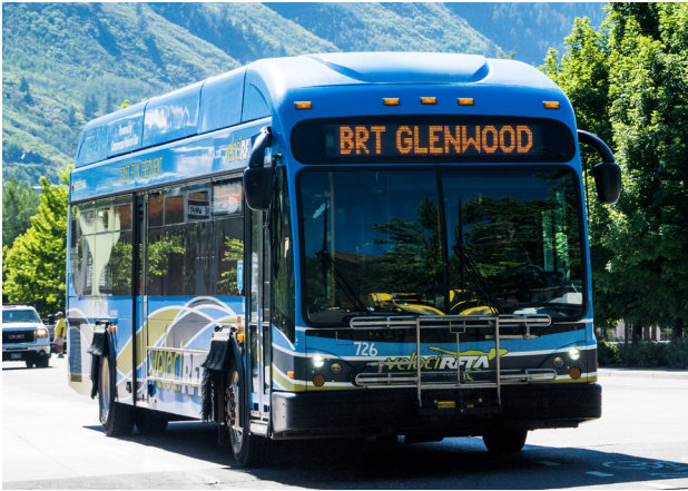
All of RFTA's valley buses have front-load racks. Bikes on the two/three capacity racks are lifted and placed into wheel slots.
